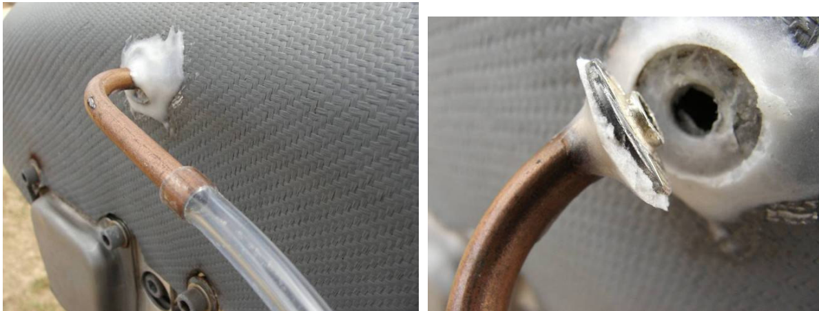
Figure 61: Ram Air duct pressure tapping.
