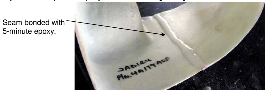
Figure 52. Ram Air Duct Front Seam
