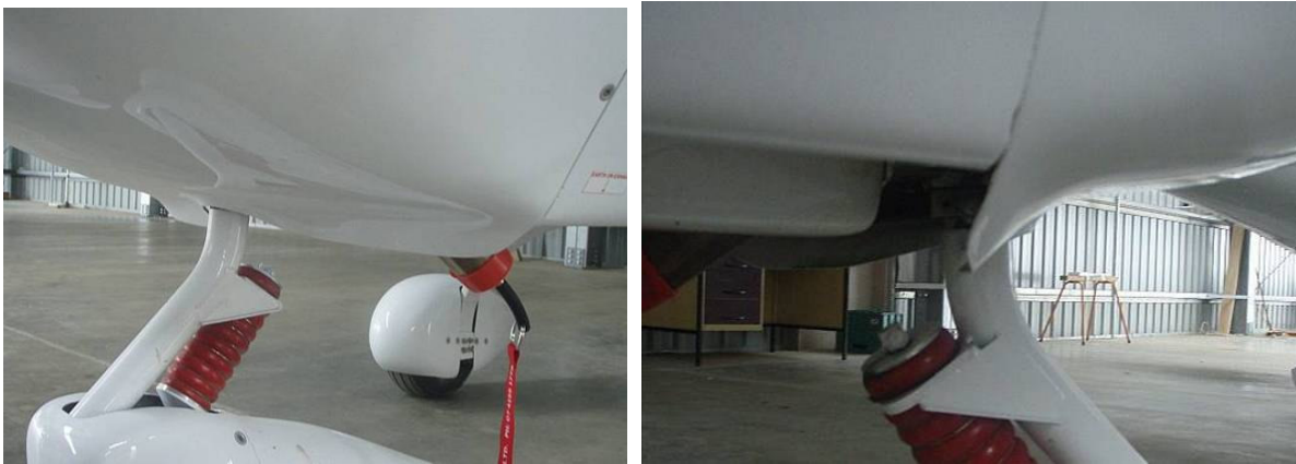
Figure 56: Lip to aid cooling as installed on a Jabiru.
