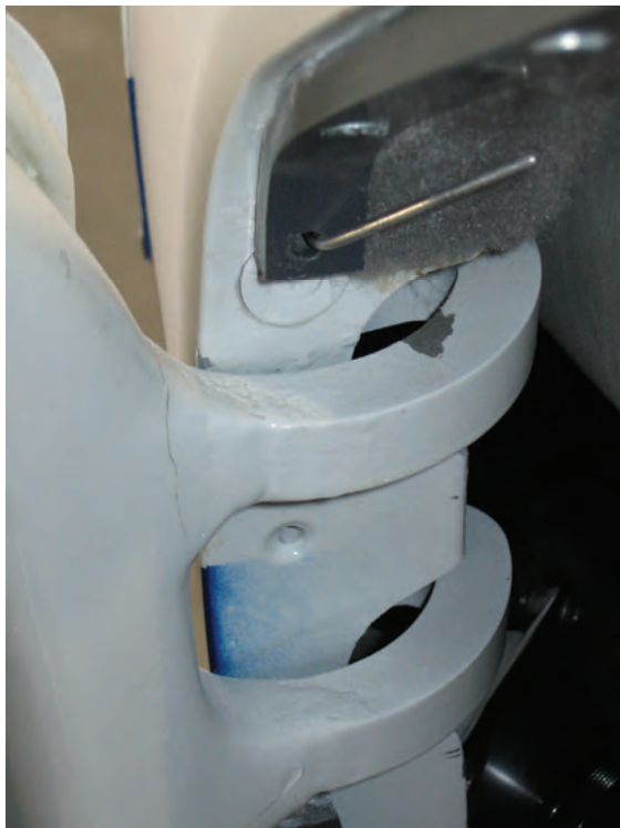
Figure 3-6: "Old" style door hinge, pilot's side.
