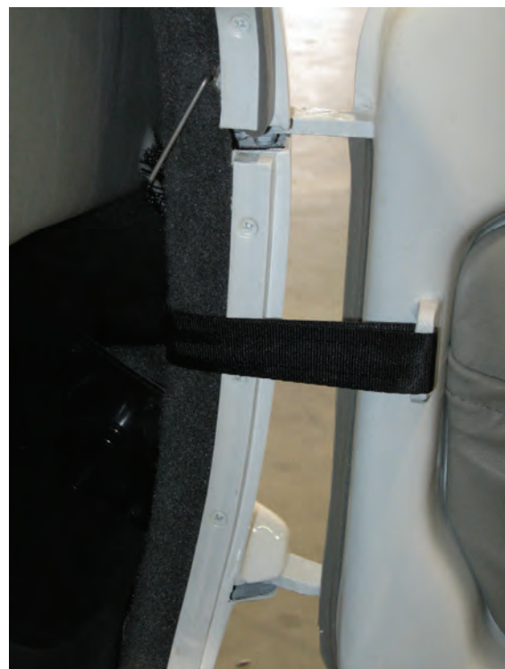
Figure 3-7: "New" style door hinge, passenger side.
