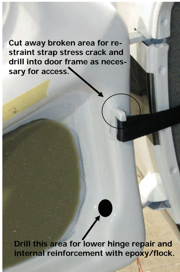
Figure 12-1: Hinge repair
