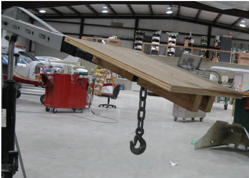
Figure 2-2: Plywood Jacking Platform on Engine Hoist
