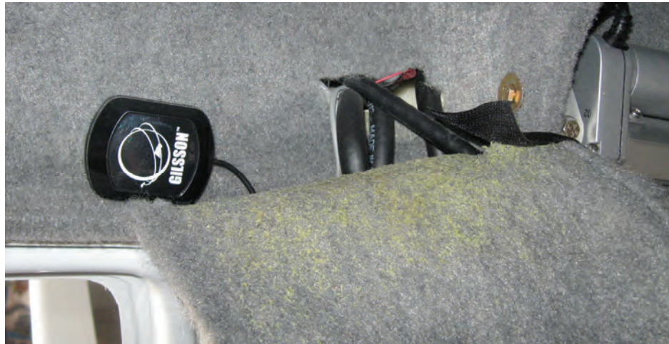
Figure 11-5: GPS Antenna head, over-door location. Door post cover peeled back for clarity.
