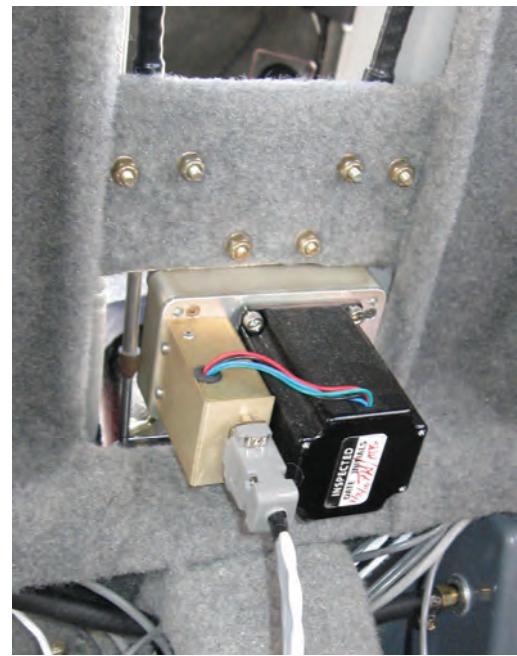
Figure 11-7: Autopilot servos. Pitch servo installation, all years (top left). New style roll servo viewed from front, between seats (top right). New style roll servo installation from rear (bottom right). Old style roll servo installation (bottom left).
