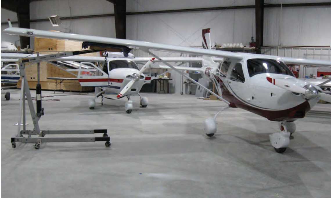
Figure 2-3: Jacking Aircraft with Engine Hoist
