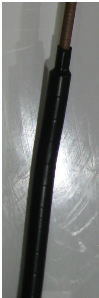
Figure 11-6: Ferrite baluns sealed onto antenna cable with heat-shrink tubing (left) and finished antenna wiring showing double-holed balun (right).
