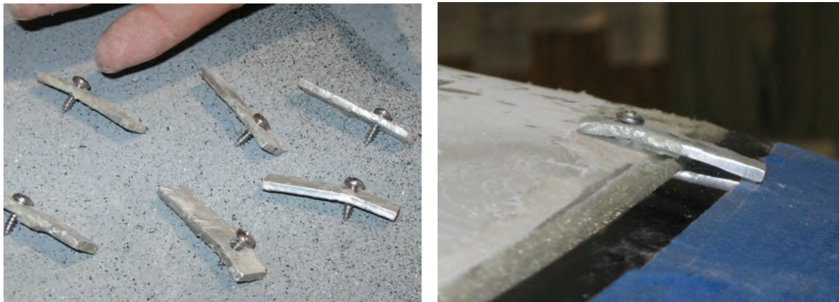
Figure 3-1: Window clamps made from 0.125" aluminum stock and sheet metal screws (left). Clamp in position holding upper portion of windshield to fuselage (right).
