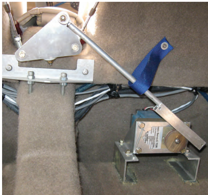
Figure 11-7: Autopilot servos. Pitch servo installation, all years (top left). New style roll servo viewed from front, between seats (top right). New style roll servo installation from rear (bottom right). Old style roll servo installation (bottom left).
