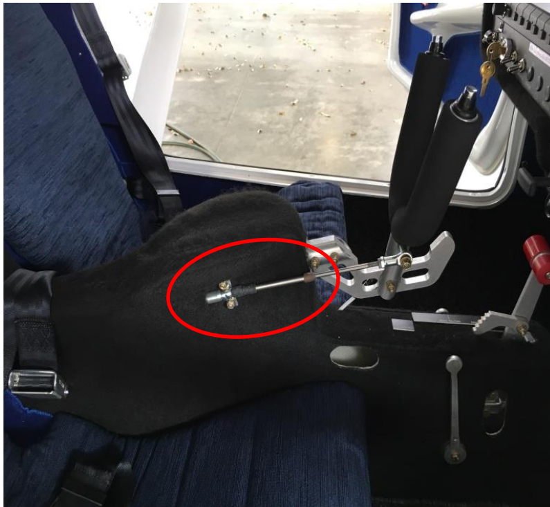
Figure 3 – Location of cables to inspect
