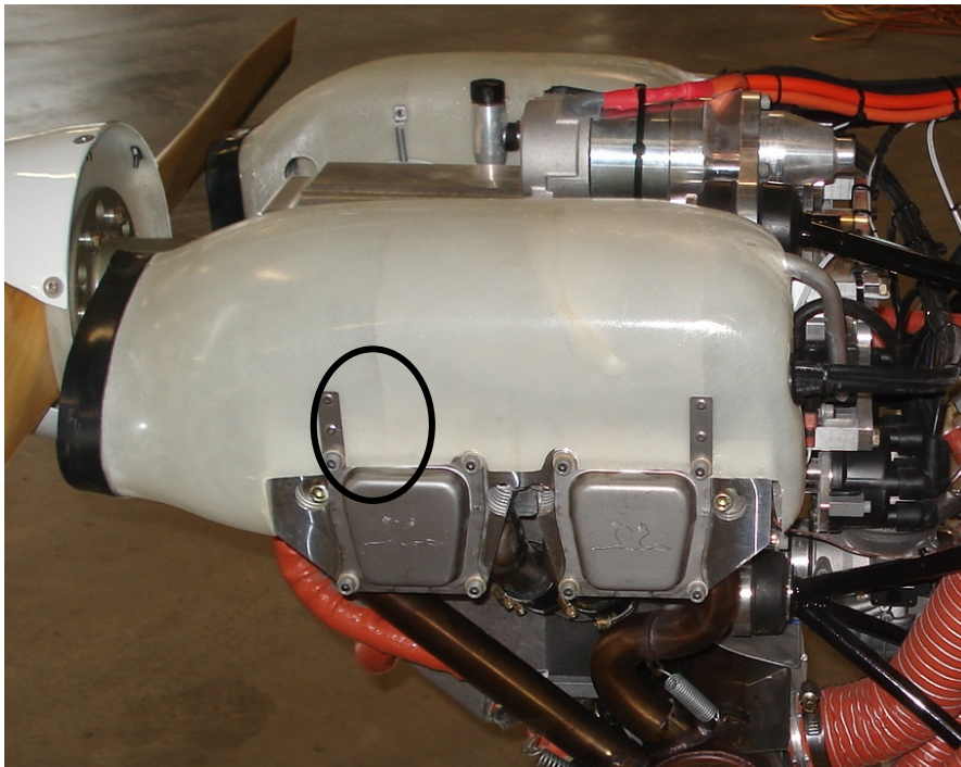
Figure 93 – Air Duct Hard Point Reinforcement
