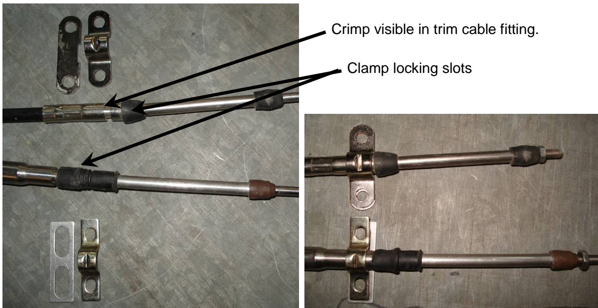
Figure 61 – Cable & Clamp Comparison
