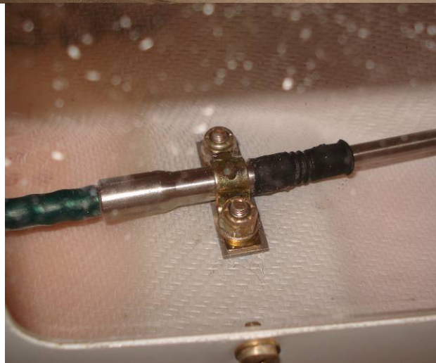
Figure 59 – Clamp Installations (Elevator & Aileron)
