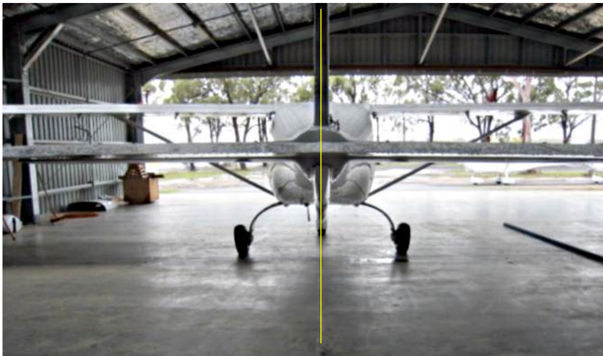
Figure 17 – Wheel Alignment Set Up
