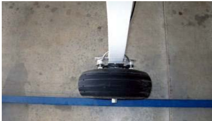
Figure 18 – Alignment Straight Edge In Position
