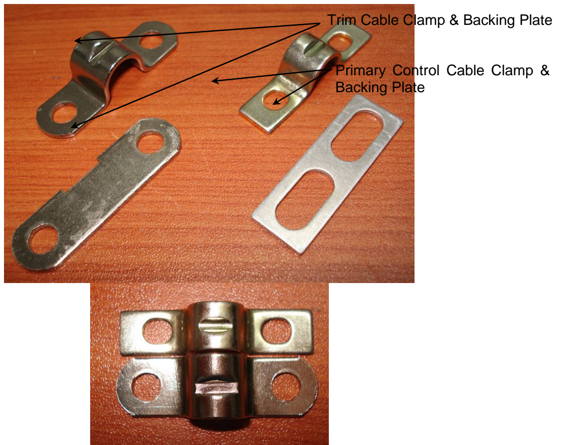
Figure 57 – Clamp Comparison (Primary Cable Clamp Upper on Right Picture)
