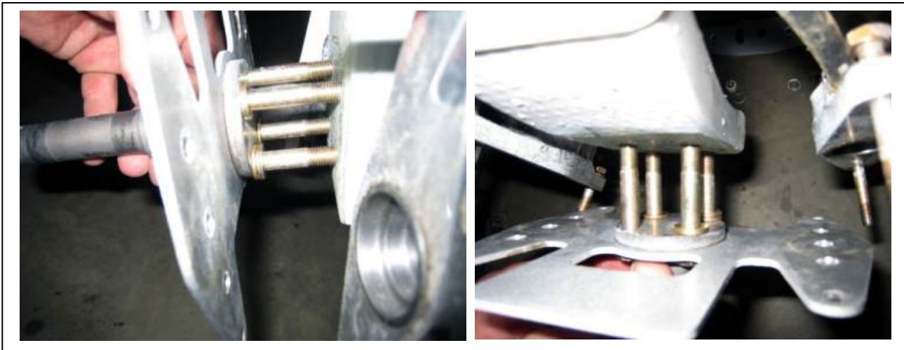
Figure 20 – Camber / Toe-In Adjustment
